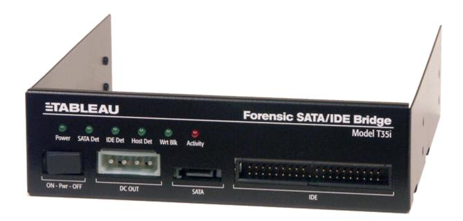
The T35i is designed to mount directly in a forensic workstation. Internally the T35i connects to the workstation through a high-performance FireWire800 connection. Externally, the T35i can be connected to SATA or IDE hard disks (one at a time) for write-blocked forensic acquisitions.
